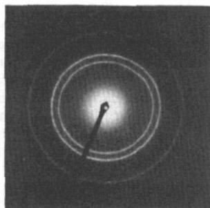
Figure 1. The electron diffraction pattern of the carbide phase formed in the Cr thin films after ion implantation to a dose of 2.5 \times 10^{17} \text{ cm}^{-2} . Similar patterns were also observed in the Ti and V systems.
